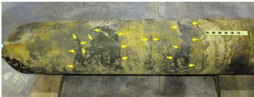
**Figure 8.** Underside of pipe upstream of rupture exhibiting primarily uncoated pipe. Boundaries of uncoated portion of pipe are indicated by yellow arrows.
