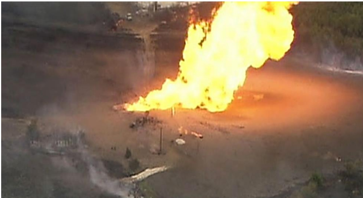
Figure 1. Natural gas burning from 36-inch-diameter Enterprise pipeline
