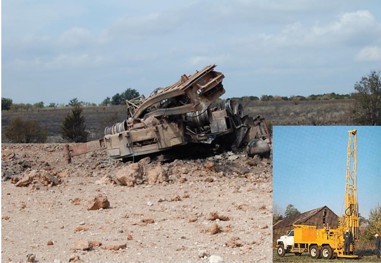
Figure 4. Upside-down, 60-ton C&H auger truck; exemplar truck shown in lower right
