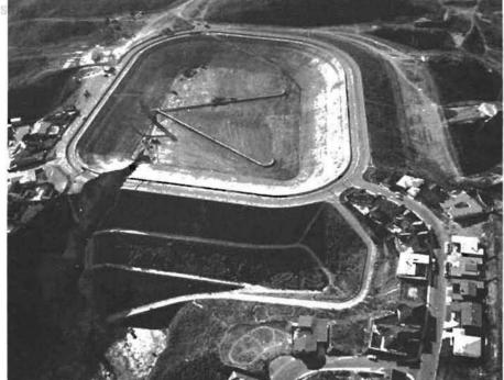
Fig. 2-1. Baldwin Hills Reservoir after failure.
