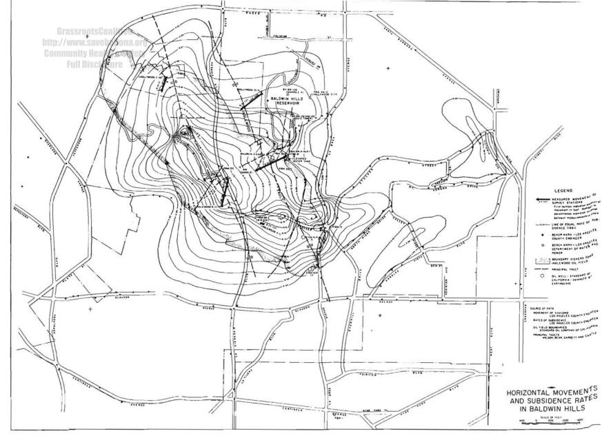
Fig. 2.4 Horizontal movements and subsidence rates in Baldwin Hills
