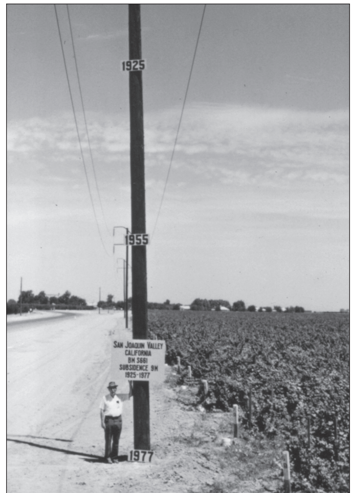
Figure 4. Approximate point of maximum subsidence in the San Joaquin Valley, California. Land surface subsided ~9 m from 1925 to 1977 due to aquifer-system compaction. Signs on the telephone pole indicate the former elevations of the land surface in 1925 and 1955. Photograph by Richard Ireland.
